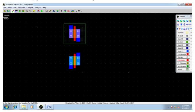
4. Select Polysilicon from the Palette and connect the gate of PMOS and NMOS.
