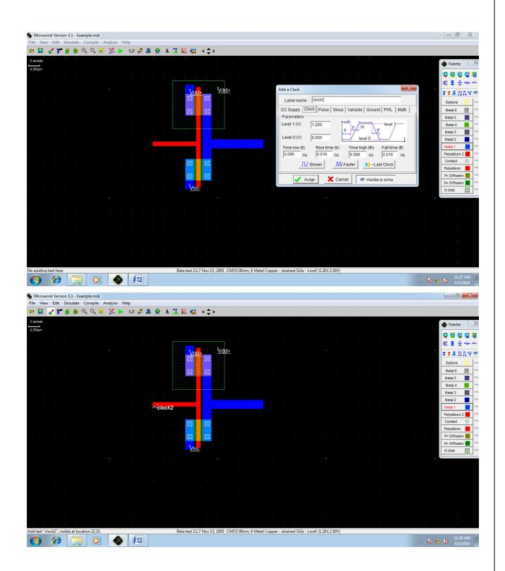
9. Now output is placed by choosing Visible node symbol from the Palette and click assign to place it at the output port.
