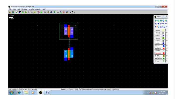
5. Now Connect the two transistors using a metal1 layer from the Palette.
