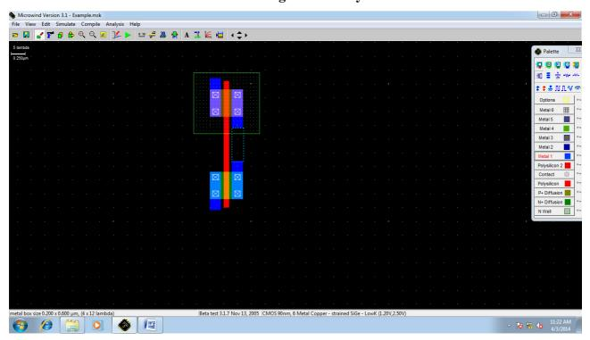
6. Now make connections for input and output using corresponding layers.
