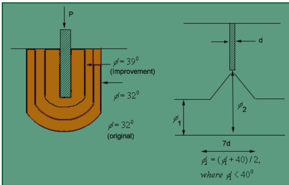
Fig.5.4b Improvement in  $f$  due to pile driving
